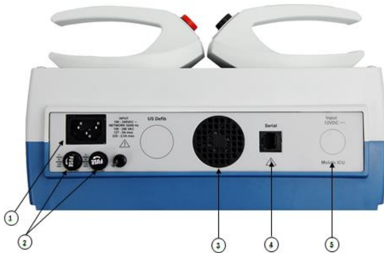
Image26 - CARDIOSTART DEFIBRILLATOR MONITOR Parts Identification – Side and Rear View
