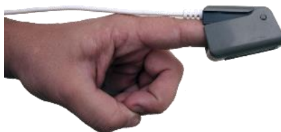
Image33 - Oximetry sensor positioning.
